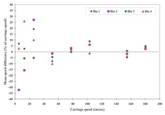
Fig. A1 Mean speed differences of ADP s33/500 KHz unit (6/17/99)
