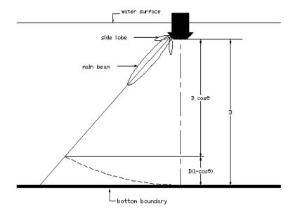
Fig. 4a Profile depth lost due to sidelobe contamination near the boundary
