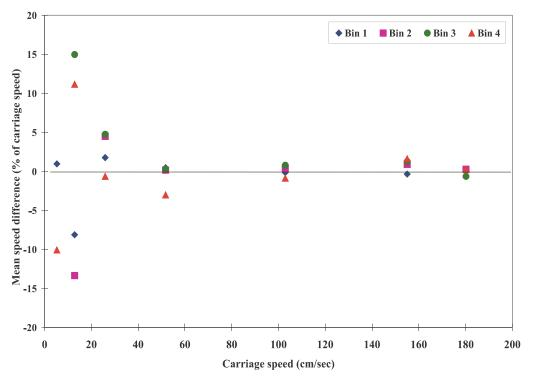
Fig. A3 Mean speed differences of ADCP r849/600 KHz unit (6/22/99)
