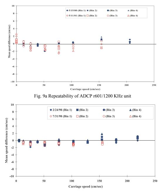
Fig. 9b Repeatability of ADCP r604/1200 KHz unit
