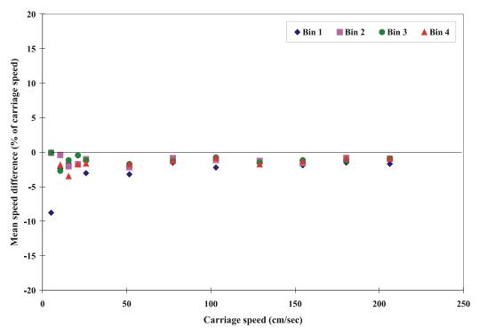
Fig. A11 Mean speed differences of ADCP r135/1200 KHz unit (9/5/96)
