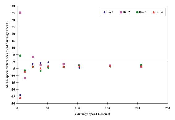
Fig. A21a Mean speed differences of ADP s4032/1500 KHz unit (4/16/98)
