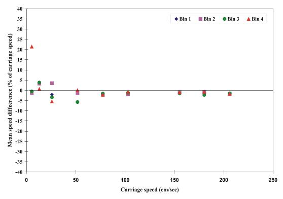
Fig. A18 Mean speed differences of ADP s53/1500 KHz unit (6/22/99)
