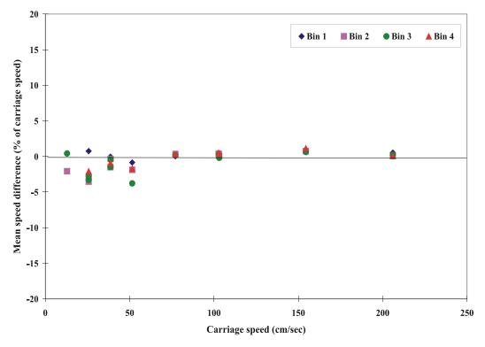
Fig. A13a Mean speed differences of ADCP r601/1200 KHz unit (5/15/00)
