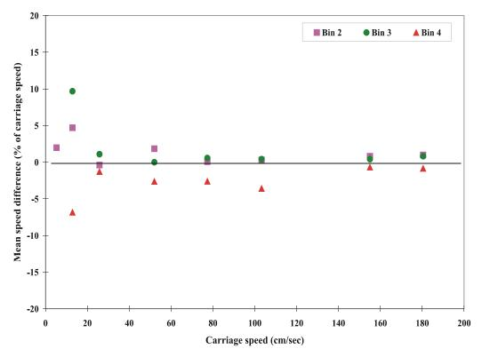
Fig. A8 Mean speed differences of ADCP r949/600 KHz unit (6/16/99)
