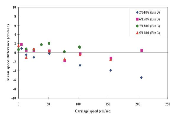
Fig. 9f Repeatability of ADP s4033/1500 KHz unit
