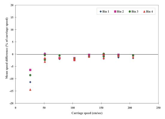
Fig. A12 Mean speed differences of ADCP r523/1200 KHz unit (4/6/95)
