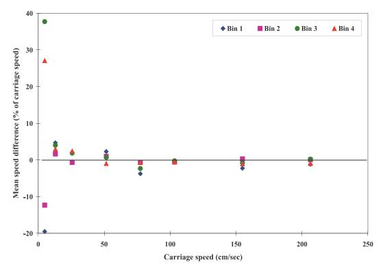
Fig. A22b Mean speed differences of ADP s4033/1500 KHz unit (6/15/99)
