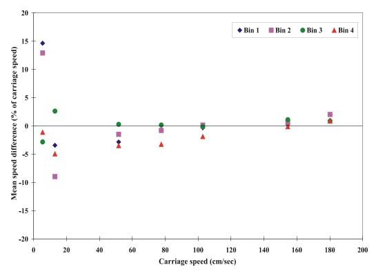
Fig. 6b Mean speed differences of ADCP r948/600 KHz unit (6/17/99)
