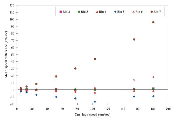
Fig. 14a Example of bin velocities affected by bottom boundary (ADCP 600 KHz)
