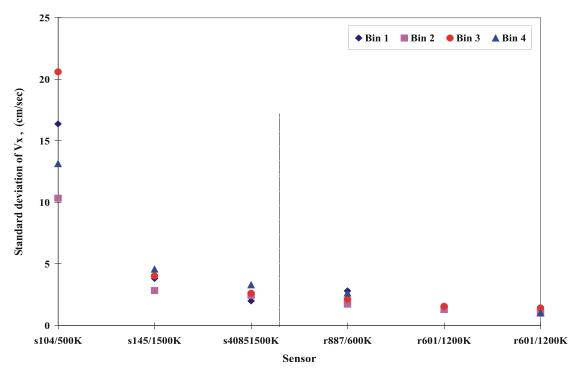
Fig. 10b Standard deviation of sensor readings at zero carriage speed
