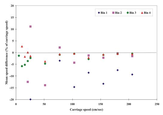
Fig. A10 Mean speed differences of ADCP r134/1200 KHz unit (9/5/96)
