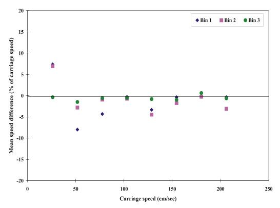
Fig. A2 Mean speed differences of ADP s4114/500 KHz unit (11/19/96)
