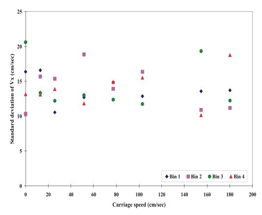
Fig. 7a Standard deviation of velocity component for ADP s104/500 KHz unit (9/14/99)
