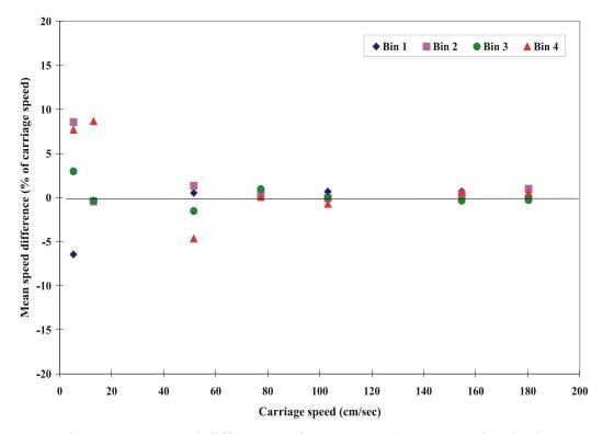
Fig. A4 Mean speed differences of ADCP r886/600 KHz unit (6/16/99)
