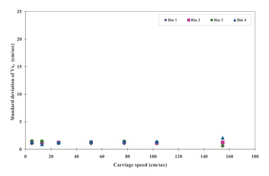
Fig. 7c Standard deviation of velocity component for ADCP r238/1200 KHz unit (6/17/99)
