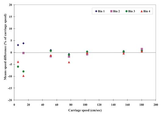
Fig. A7 Mean speed differences of ADCP r944/600 KHz unit (6/16/99)
