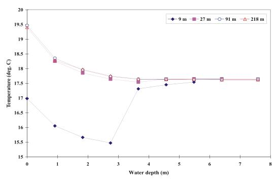
Fig. 11 Sample temperature distribution in the tow basin
