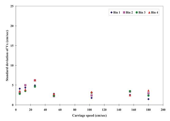
Fig. A27 Standard deviation of velocity component for ADCP r849/600 KHz unit (6/22/99)
