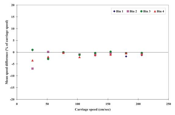
Fig. A26a Mean speed differences of ADP s4126/1500 KHz unit (11/19/96)
