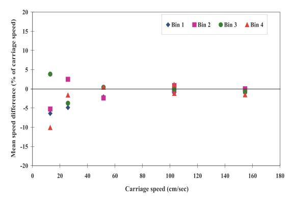
Fig. A20 Mean speed differences of ADP s312/1500 KHz unit (5/11/01)
