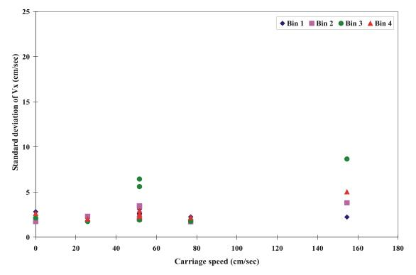
Fig. A28 Standard deviation of velocity component for ADCP r887/600 KHz unit (5/12/99)
