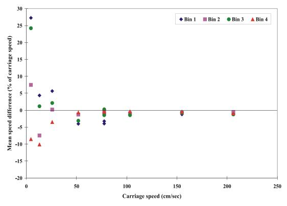
Fig. A21b Mean speed differences of ADP s4032/1500 KHz unit (6/15/99)
