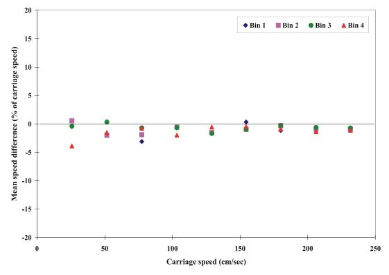
Fig. A24a Mean speed differences of ADP s4123/1500 KHz unit (11/19/96)
