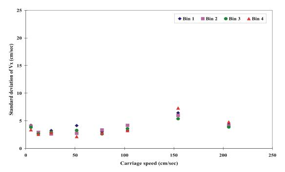
Fig. A32 Standard deviation of velocity component forADP s4033/1500 KHz unit (2/24/98)
