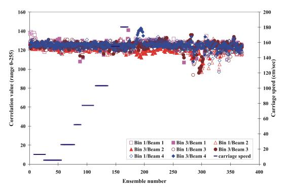
Fig. 13c Example of correlation value associated with non-uniform backscatter distribution (ADCP r949/600 KHz, 6/16/99, Bin 1 empty)
