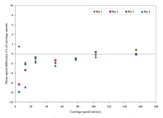
Fig. 6c Mean speed differences of ADCP r238/1200 KHz unit (6/17/99)
