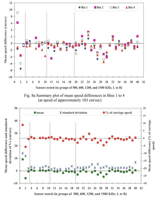
Fig. 8b Summary plot of mean speed differences and standard deviation of Vx (Bin 3, at speed of approximately 103 cm/sec)
