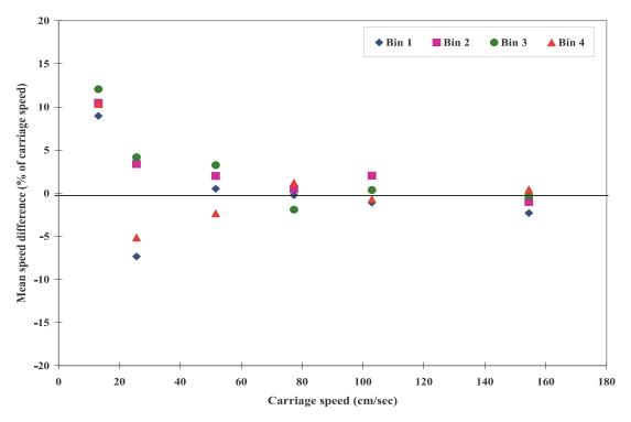
Fig. A26b Mean speed differences of ADP s4126/1500 KHz unit (5/11/01)
