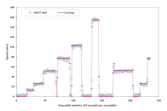
Fig. 5a Sample plot of carriage and sensor ensemble speeds (ADCP r601, Bin 3, 5/11/01)
