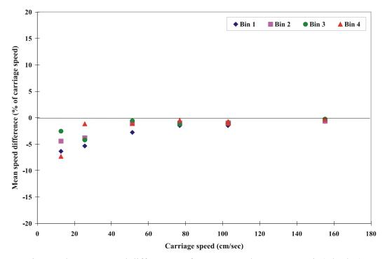
Fig. A14b Mean speed differences of ADCP r604/1200 KHz unit (7/31/98)
