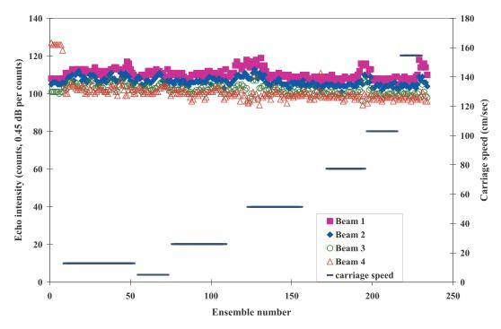
Fig. 12 Typical echo intensity data (ADCP r238/1200 KHz, 6/17/99)
