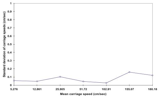
Fig. 2 Typical accuracy of carriage speed
