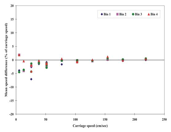
Fig. A14a Mean speed differences of ADCP r604/1200 KHz unit (2/24/98)
