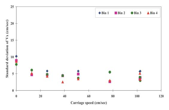
Fig. A30 Standard deviation of velocity component for ADP s21/1500 KHz unit (7/13/00)
