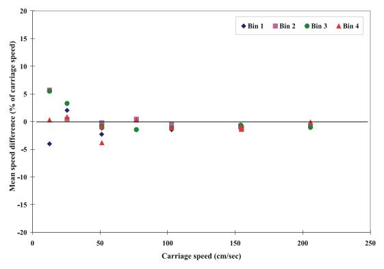
Fig. A24b Mean speed differences of ADP s4123/1500 KHz unit (7/30/98)
