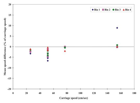
Fig. A5 Mean speed differences of ADCP r887/600 KHz unit (5/12/99)
