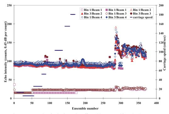
Fig. 13a Example of echo intensity affected by non-uniform backscatter distribution (ADCP r949/600 KHz, 6/16/99, Bin 1 empty)
