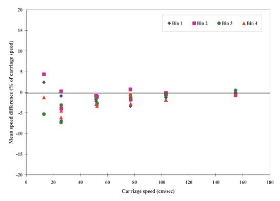
Fig. 13b Mean speed differences of ADCP r601/1200 KHz unit (5/11/01)
