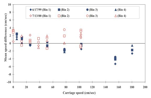
Fig. 9d Repeatability of ADP s21/1500 KHz unit
