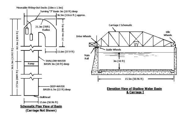
Fig. 1a Towing basin and earriage 1
