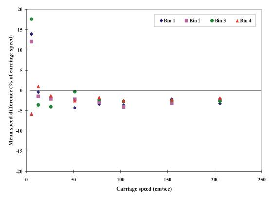
Fig. A22a Mean speed differences of ADP s4033/1500 KHz unit (2/24/98)
