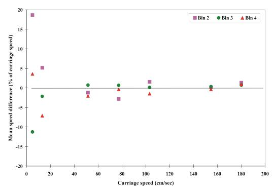
Fig. A6 Mean speed differences of ADCP r942/600 KHz unit (6/16/99)
