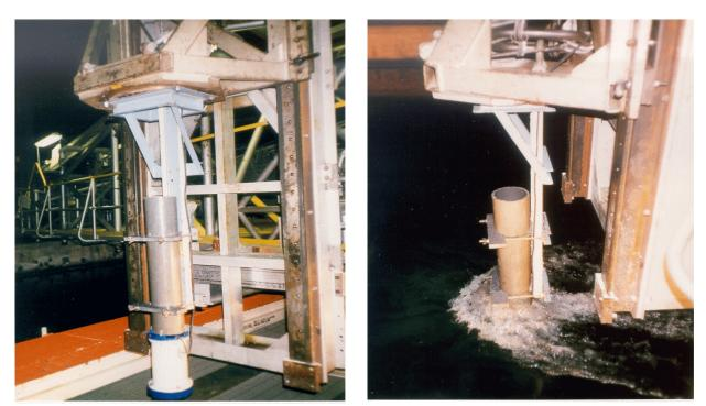
Fig. 3a Mounting of sensor on the carriage
