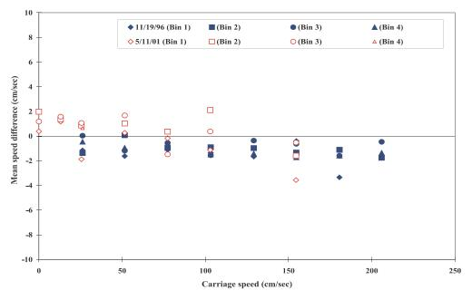
Fig. 9i Repeatability of ADP s4126/1500 KHz unit
