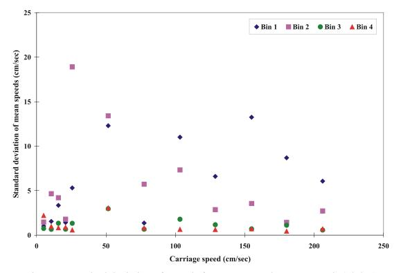
Fig. A29 Standard deviation of speeds for ADCP r134/1200 KHz unit (9/5/96)
