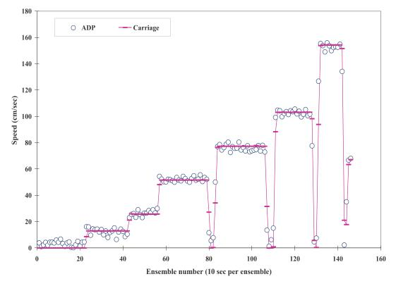
Fig. 5b Sample plot of carriage and sensor ensemble speeds (ADP s4033, Bin 3, 5/11/01)
