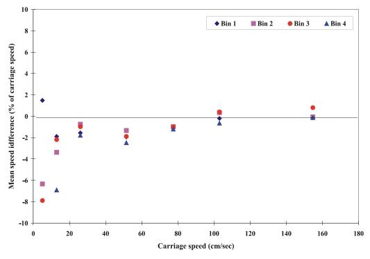
Fig. 6d Mean speed differences of ADP s20/1500 KHz unit (9/8/97)
