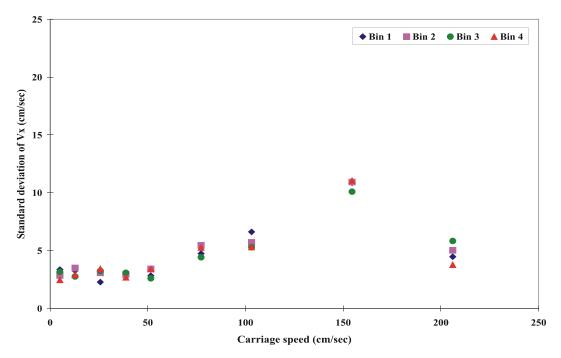
Fig. A31 Standard deviation of velocity component for ADP s4032/1500 KHz unit (4/16/98)
