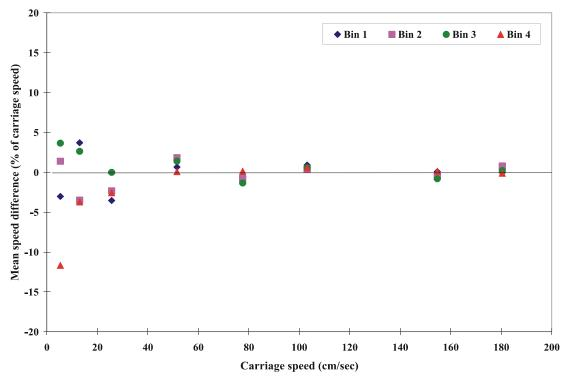
Fig. A25b Mean speed differences of ADP s4125/1500 KHz unit (11/19/96)
