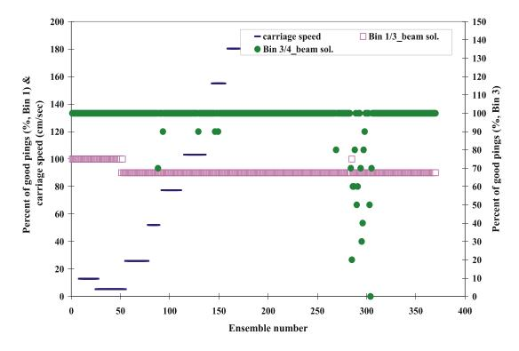
Fig. 13b Example of percent of good pings associated with non-uniform backscatter distribution (ADCP r949/600 KHz, 6/16/99, Bin 1 empty)
