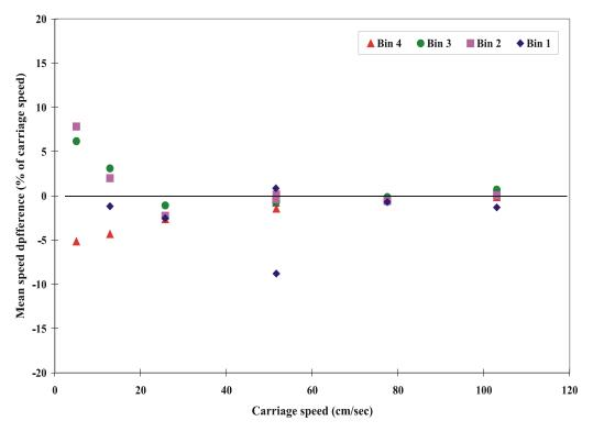
Fig. A9 Mean speed differences of ADCP r113/1200 KHz unit (6/16/99)
