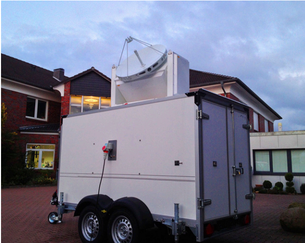
FIG. 3. The MIRA-35 cloud radar with the scanning unit at METEK GmbH. The photo was provided by METEK GmbH.
