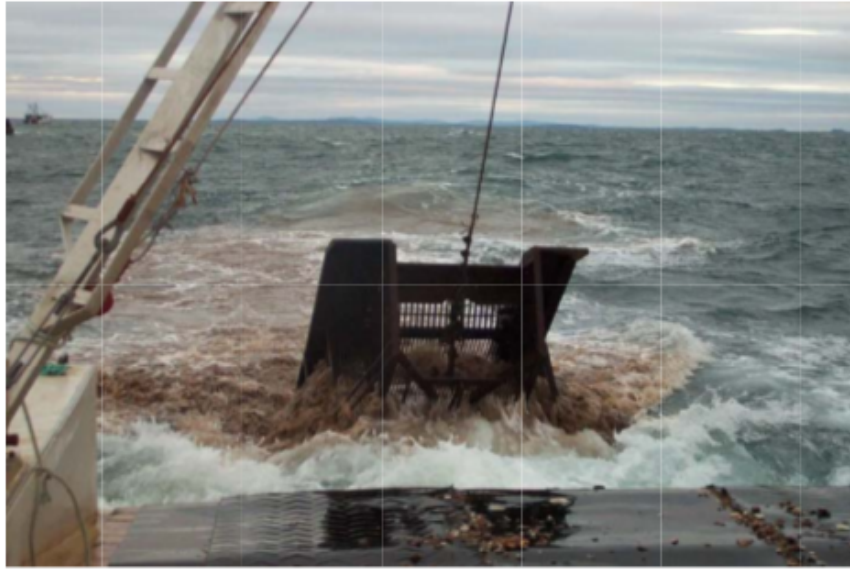
Figure 235: After being brought to the surface, the catch is washed and mud rinsed away in the propeller wash of the survey vessel.
