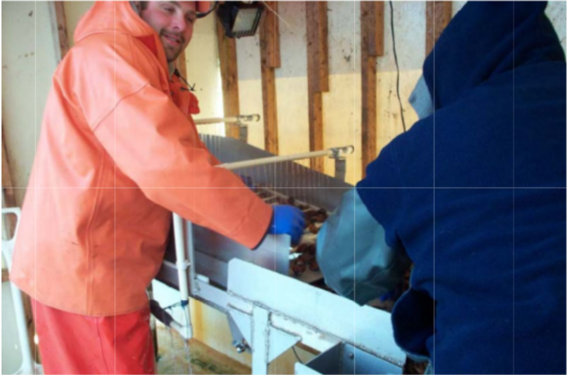
Figure 237: Processing the survey catch on shaker table, used to remove shell fragments and mud. This step is performed in commercial operations as well.
