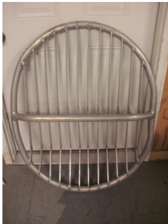
Figure 1. Curved bottom flat-bar TED with 2-inch bar spacing. Bars made from 0.25-inch x 1.5 inch aluminum flat-bar.
