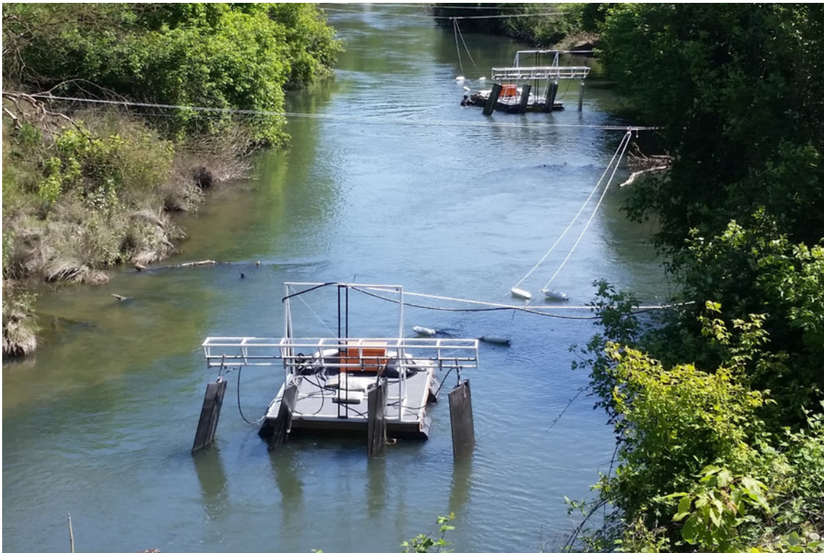
Figure 42. Raft-mounted hydrofoil arrays on the Mokelumne River.
