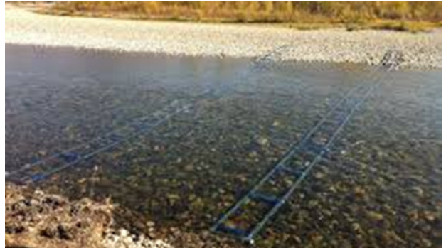
Figure 1. Examples of standard swim-through and swim-over antennas used in open stream and river channels.
