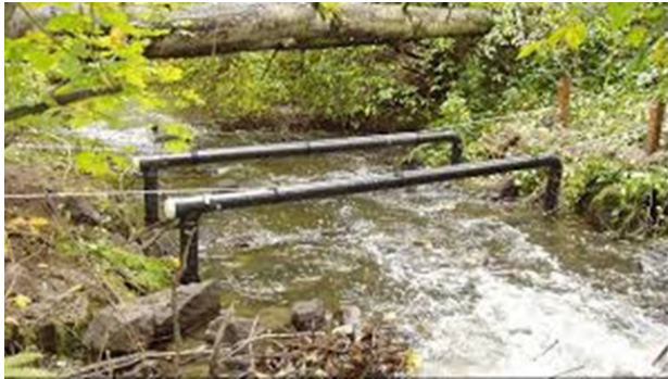
Figure 1. Examples of standard swim-through and swim-over antennas used in open stream and river channels.
