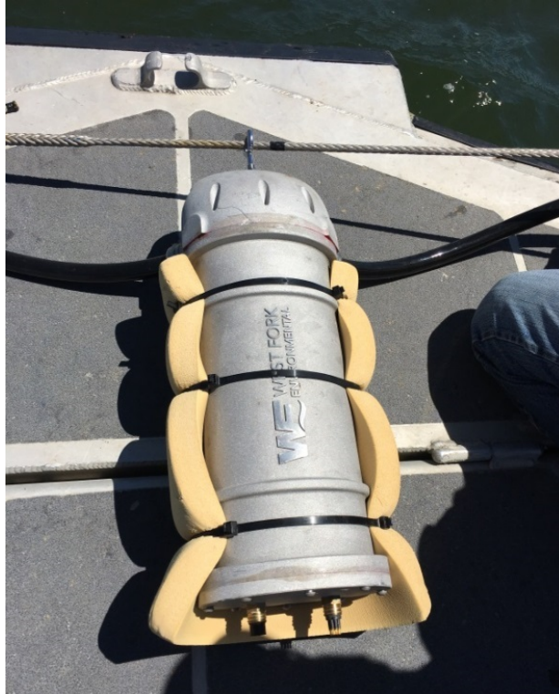
Figure D.3. Buoyancy compensation for first prototype manufactured housing.
