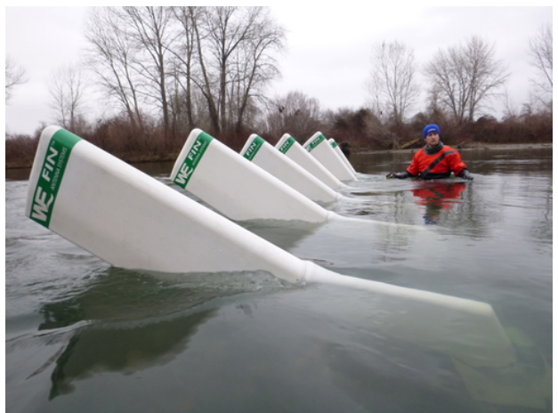
Figure 3. Recently developed antenna designs for open channels: floating mat antenna made by Biomark, and bottom-mounted vertical fin antenna made by West Fork Environmental.
