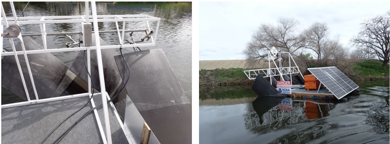
Figure 17. Rotation of the San Joaquin after several days of tidal cycles before modifications were made to stabilize orientation of the hydrofoils and position of the rafts.
