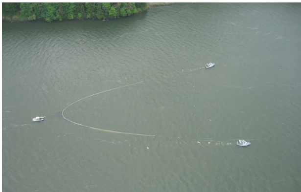
Figure 2. Towed pair-trawl antenna array used in the upper Columbia River estuary.
