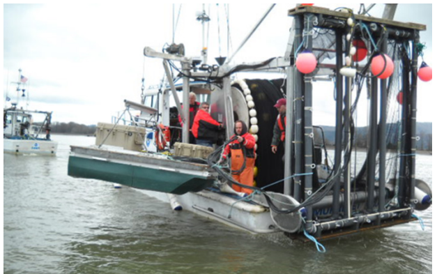
Figure 2. Towed pair-trawl antenna array used in the upper Columbia River estuary.
