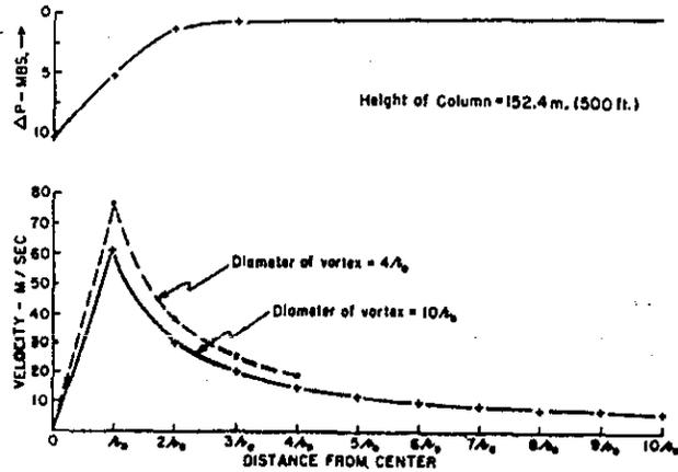
Figure 10. Calculated profile of velocity and pressure in a dust devil. The pressure profile was calculated for the case of diameter of vortex equal to  $10r_0$ . From Battan (1).
