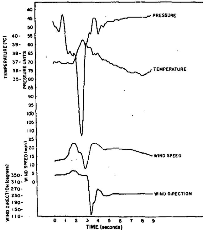
Figure 6. Temperature, pressure, and horizontal wind velocity measurements through a dust devil on July 14, 1960, 1330 MST. From Sinclair (50).
