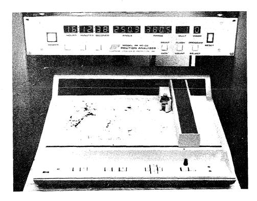
Figure 6. Position Analyzer. -9-
