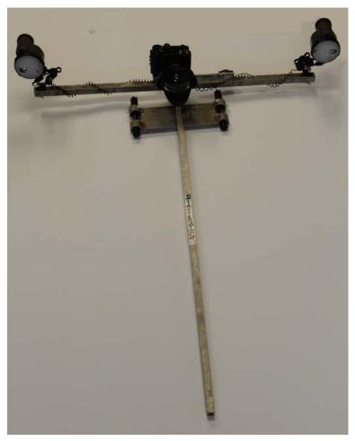
Figure 1.4. T-frame configuration. G11 Fisheye FIX® housing mounted to the frame, set at 1.5 m from the substrate, with two Inon® Z240 strobes, set 1.2 m apart.
