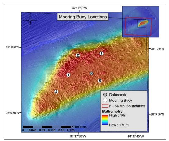
Figure 1.1. Bathymetric map of Stetson Bank showing mooring buoy locations.  $12\,$
