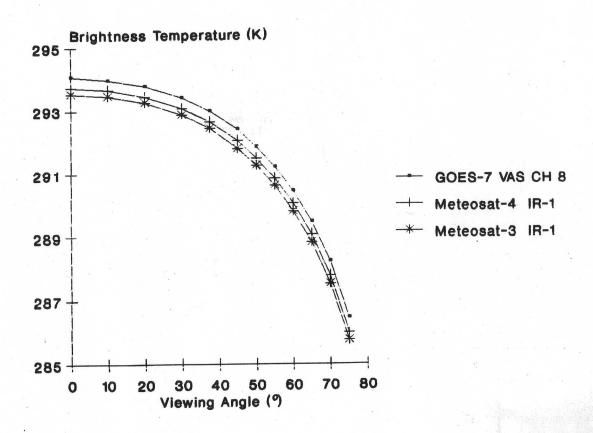
Figure 4. Brightness temperatures measured by GOES-7, Meteosat-3, and Meteosat-4 for a tropical standard atmosphere as a function of satellite viewing angle. Differences are due to the different spectral response functions of the sensors.
