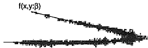
Figure 2: The principles of feature extraction. A model f with model parameter \beta is determined such that for a particular value of \beta there is a good correspondence between the model and the trace. Feature extraction is the process of choosing a suitable model and determining the best value of \beta .
