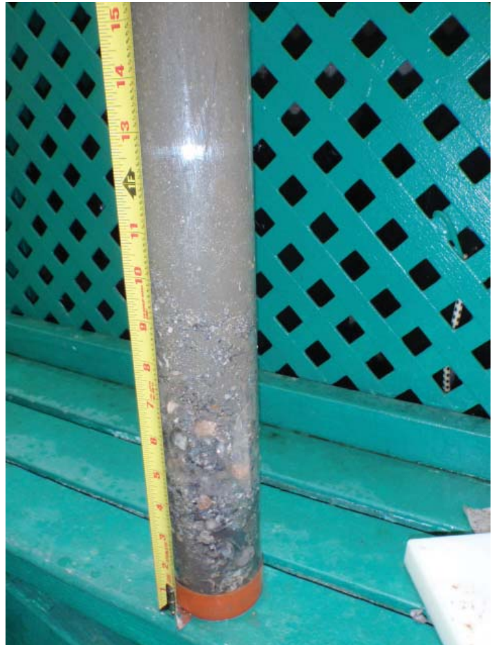
Figure 5.2. Photograph of core BB2 showing shell hash in the lower part of the core, grading to fine mud up the core in more recent sediments.
