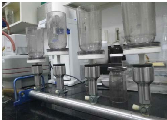
Apparatus for filtering water samples for measuring TSS in the STEER.
