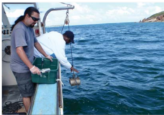
The PONAR grab used to take sediment samples in the STEER.
