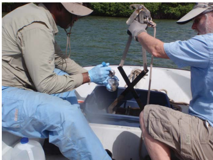
Sample of surface sediment being taken from PONAR grab by NOAA scientists.
