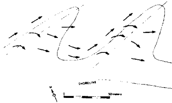
Fig. 6. Sediment transport pattern inferred from fluorescent tracer experiments.
