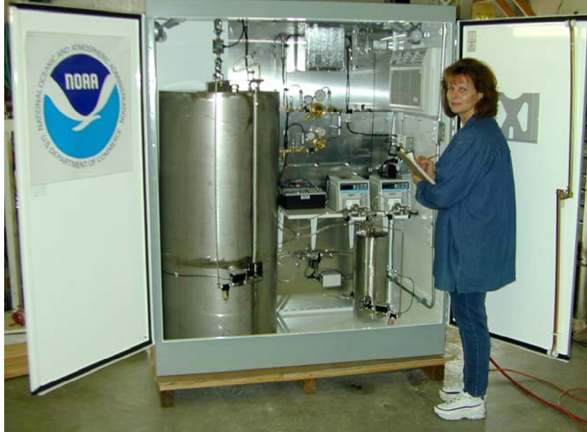
Figure 6: Release system in weather-proof cabinet.
