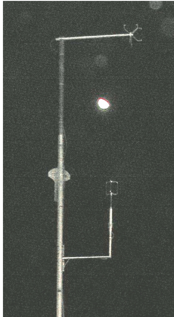
Figure 2. Sonic anemometers mounted on the LLNL mobile laboratory mast. The ATI anemometer is at the top of the mast with the GILL mounted below. A rising quarter moon can be seen between the two anemometers.
