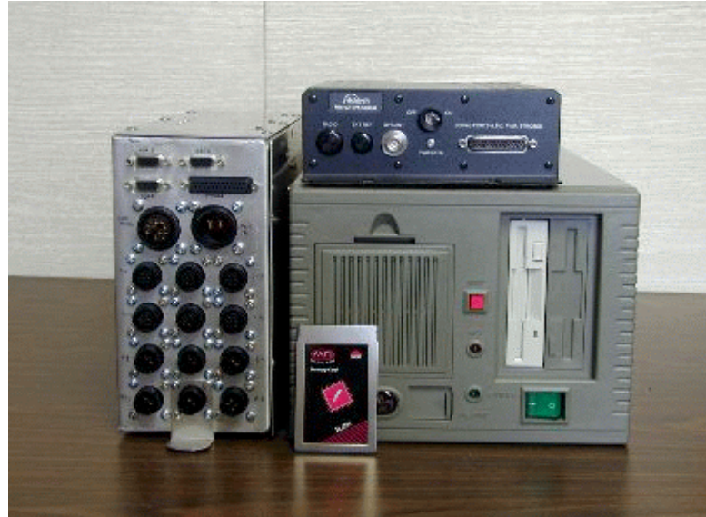
Fig. 17. N3R data acquisition PC, BAT auxiliary box, Ashtech dual-frequency GPS, and PCMCIA flash disk.
