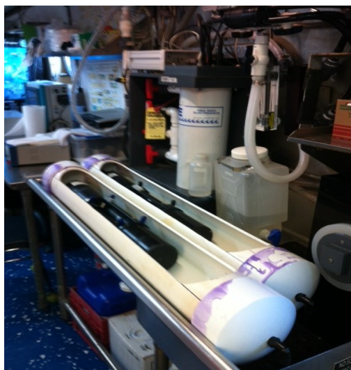
Figure 20. IOP setup shows water bath setup using the two ac-s instruments, which were located inside the PVC containers immersed in a temperature regulated water bath.
