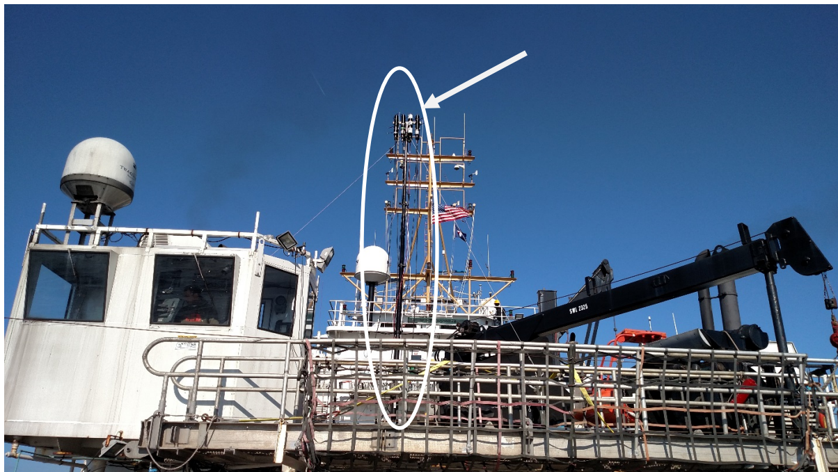
Figure 4. Telescoping tower with E_s reference sensors.
