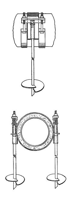
Figure 4. PIPELINE ANCHORING SYSTEM
