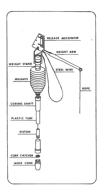
Figure 3. PISTON GRAVITY CORER
