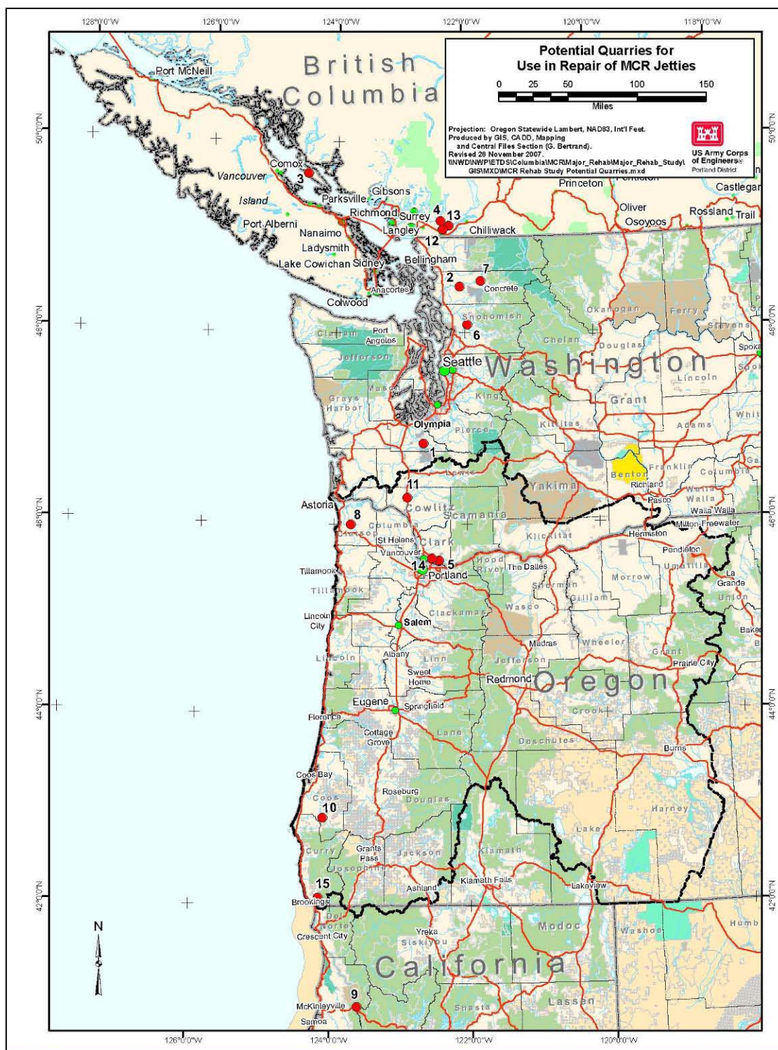
Figure 37. Potential Quarry Locations (red dots) for Repairs to MCR Jetties
