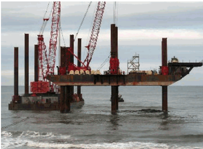
Figure 42. Illustration of a Jack-up Barge
