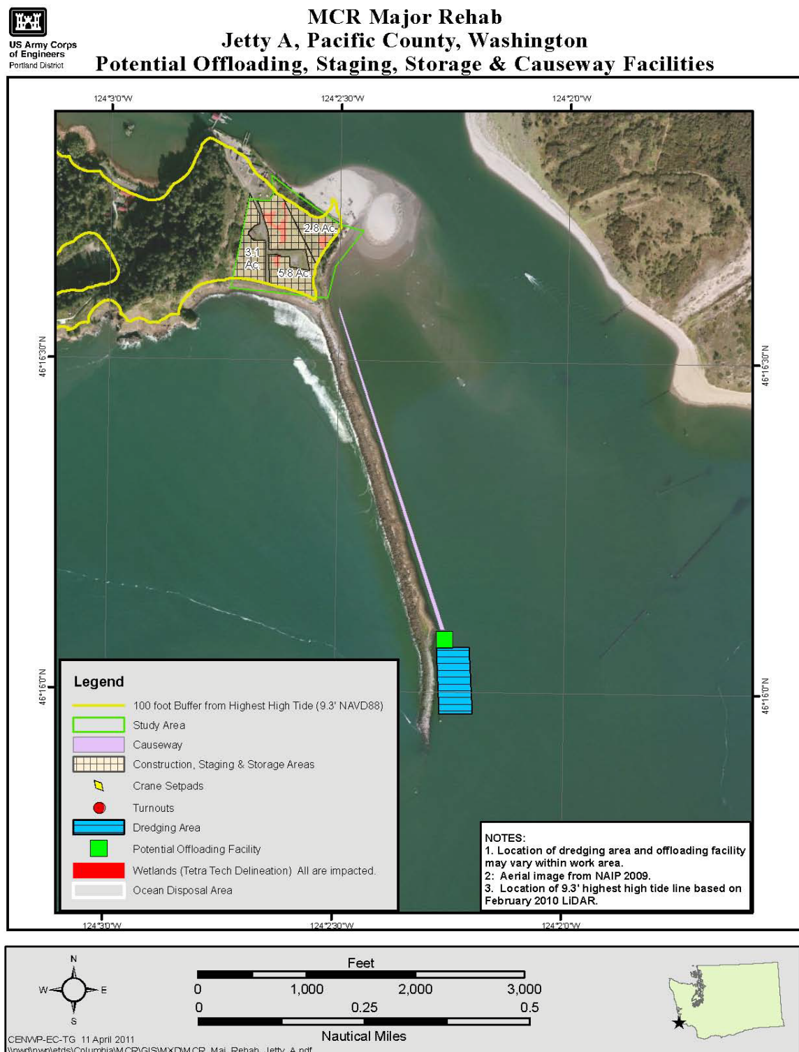
Figure 40. Jetty A Offloading, Staging, Storage and Causeway Facilities
