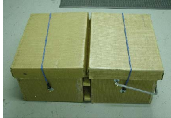
Figure A-8. PIGS control or blank sampler with the covers on and bungee cords in place.
