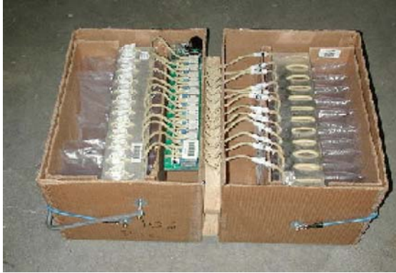
Figure A-7. PIGS control or blank sampler showing source cartridge (right) and receiver cartridge (left).
