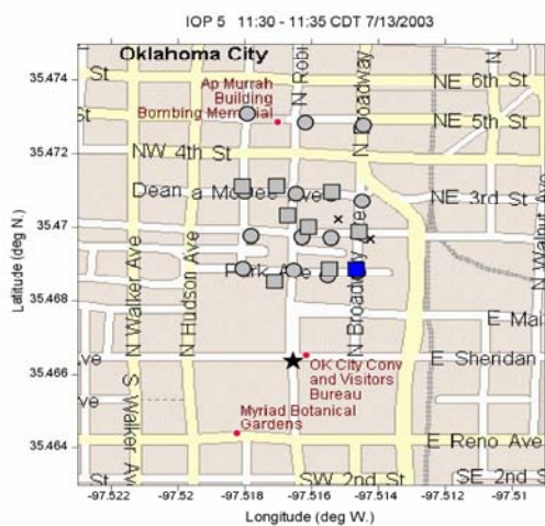
Figure I-17. CBD Super PIGS SF 6 tracer concentration footprints during IOP 5 from 0950-1000 and 1100-1140 CDT. Tracer releases occurred from 0900-0930 and 1100-1130 CDT.
