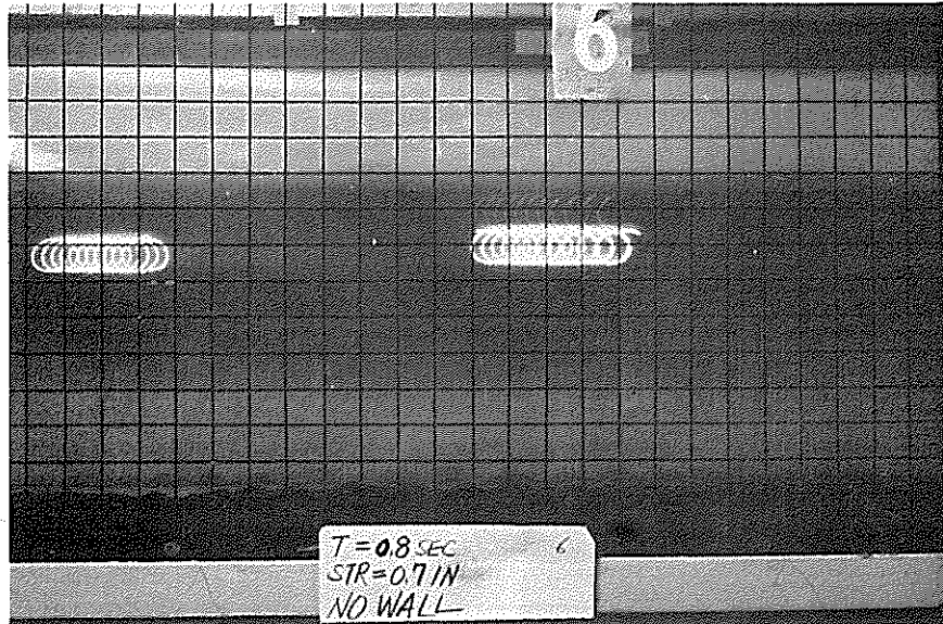
Fig. 14 PARTICLE MOTION FOR THE PROGRESSIVE WAVE CONDITION, STROKE = 0.7 IN.
