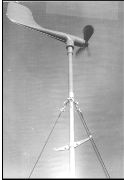
Figure 40. “Windial” installed on standard 12 foot wind support on top of the control tower. (25 October 1952). From the official station history files at the National Climatic Data Center.
