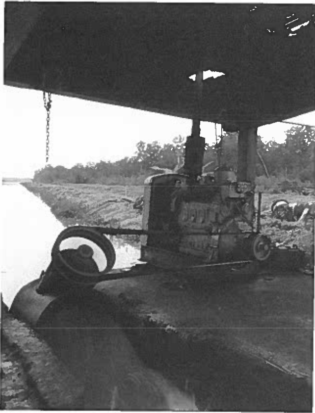
Plate 58. Increased flow rate of 61 cm axial pump during high tide when total dynamic head is reduced. Compare same flow with Plate 59.
