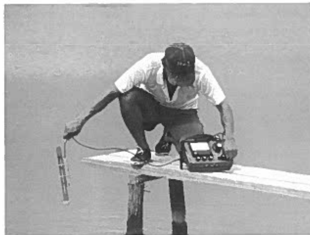
Plate 69. Extension attachment to oxygen probe and cable to ensure bottom sampling.
