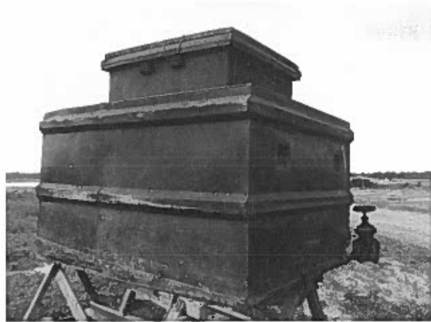
Plate 46. Juvenile transport tank with box-type neck to minimize wave action. Tank is constructed of molded polyester plastic with 1,200-liter capacity.
