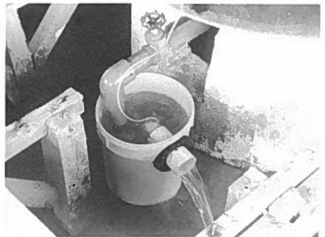
Plate 26. Acclimation tank harvest bucket in operation. Note the flow rate of bucket effluent.
