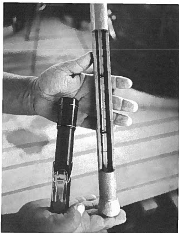
Plate 67. Glass/mercury thermometer in PVC case for protection against breakage and temperature compensated refractometer.
