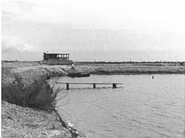
Plate 15. Pond platform station used to monitor daily parameters of secchi disk readings, near effluent weir gate. The platform should extend far enough out in the pond to have a minimum of 60 cm water depth.
