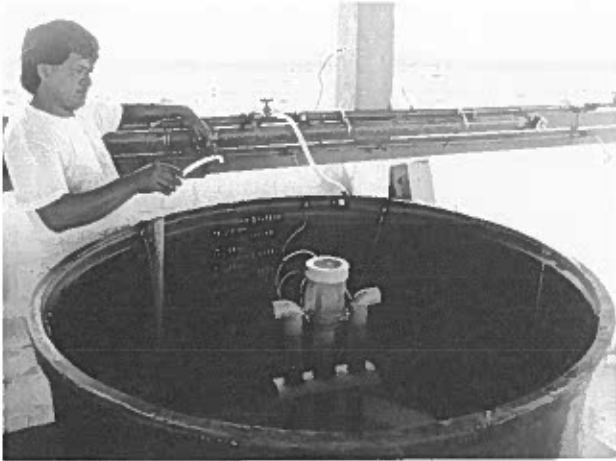
Plate 17. Empty and prepared acclimation tank. Note: 1) water inflow at the tank's bottom; 2) aeration belt at the tank-top perimeter; 3) central standpipe with aeration belt around small mesh screen; and 4) two air lift pumps parallel to the central standpipe.
