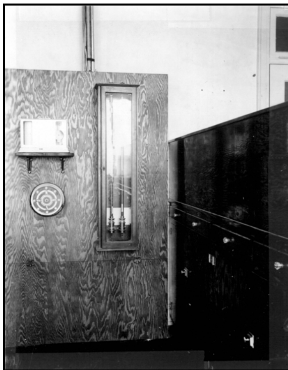
Figure 45. Barometers and barograph following the remodeling work at the Weather Bureau office at the Airport Administration Building (11 August 1943). View is east. From the official station history files at the National Climatic Data Center.
