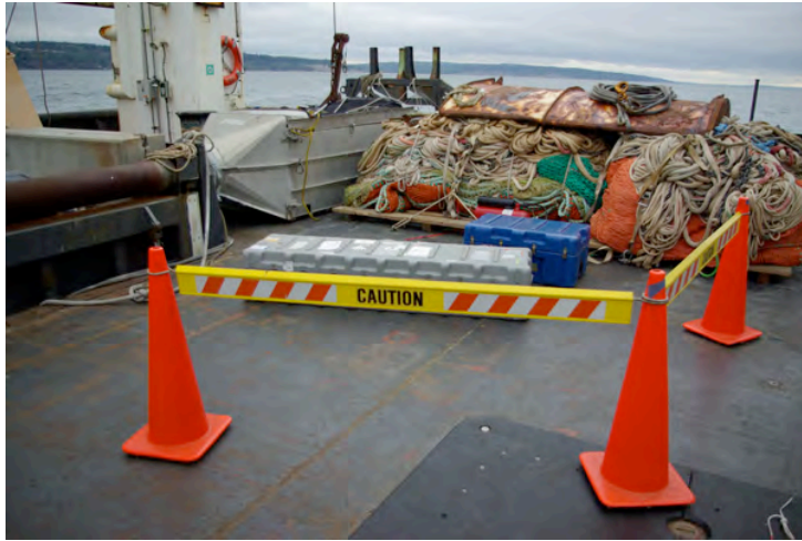
Figure 28 – Typical Cordoned Area For Fuel Operations.
