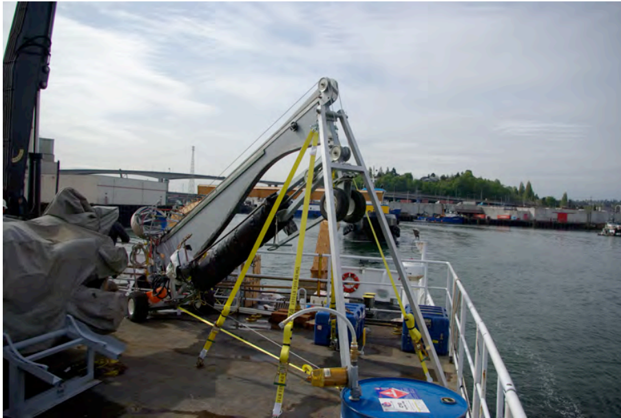
Figure 7 – Launcher Installed and Secured On The Winch Deck.
