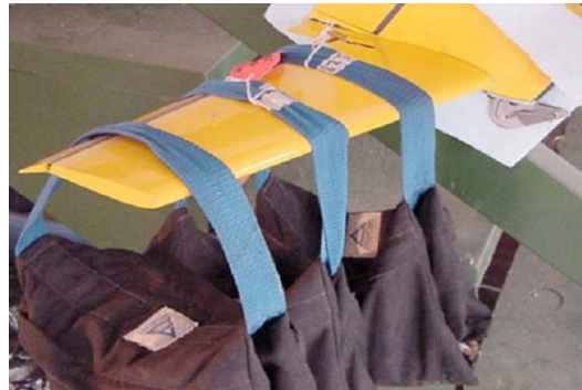
Figure 2. 20kg Static Winglet Load Test
