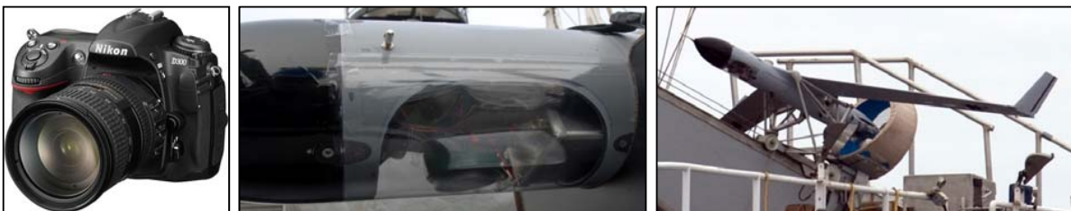
Figure 5. Nikon D300 payload mounted in downward facing ScanEagle bay.
