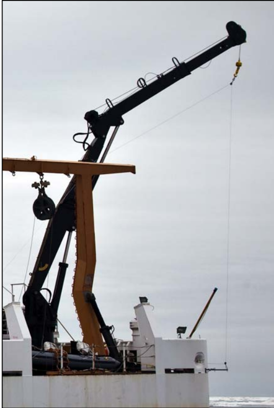
Figure 3. The SkyHook recovery system is composed of a line suspended between the ship's crane and a lower boom.
