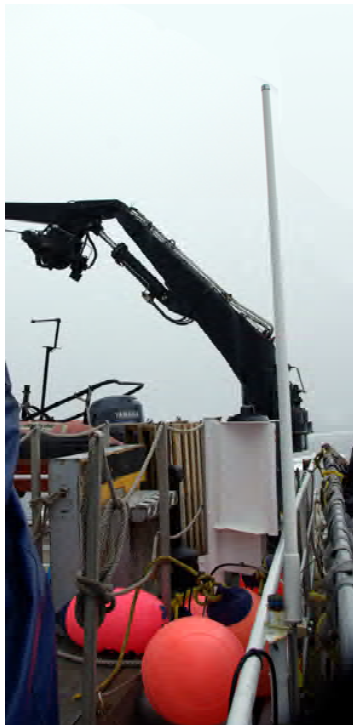
Figure 19 – Omni Directional Antenna Mounted on Ship's Railing.
