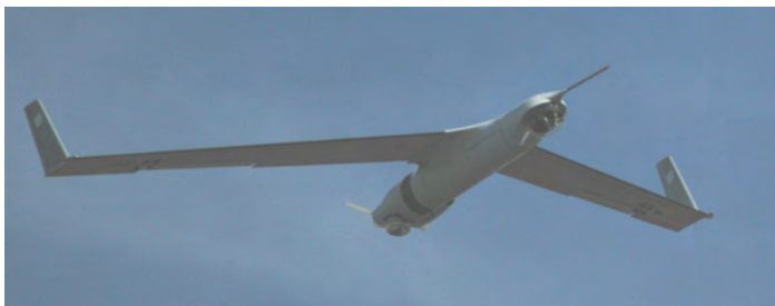
Figure 2 - Insight UAS carrying an electro-optical (visible light) analog (video) camera.
