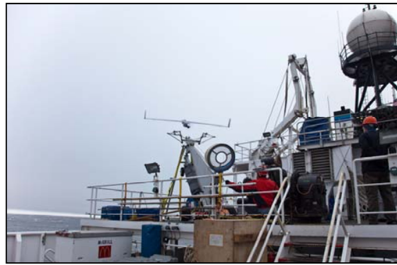
Figure 2. ScanEagle unmanned aircraft launched by pneumatic catapult from the winch deck of the NOAA ship McArthur II .
