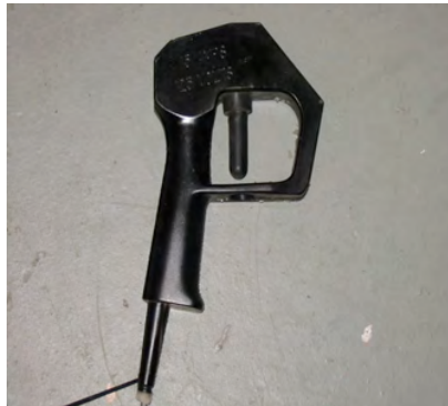
Figure 26 – the Clear-To-Land Switch.
