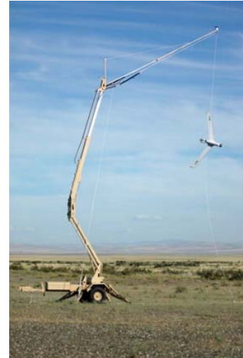
Figure 12. Skyhook Recovery System
