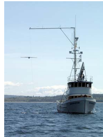
Figure 13. SkyHook Installed Aboard Ship
