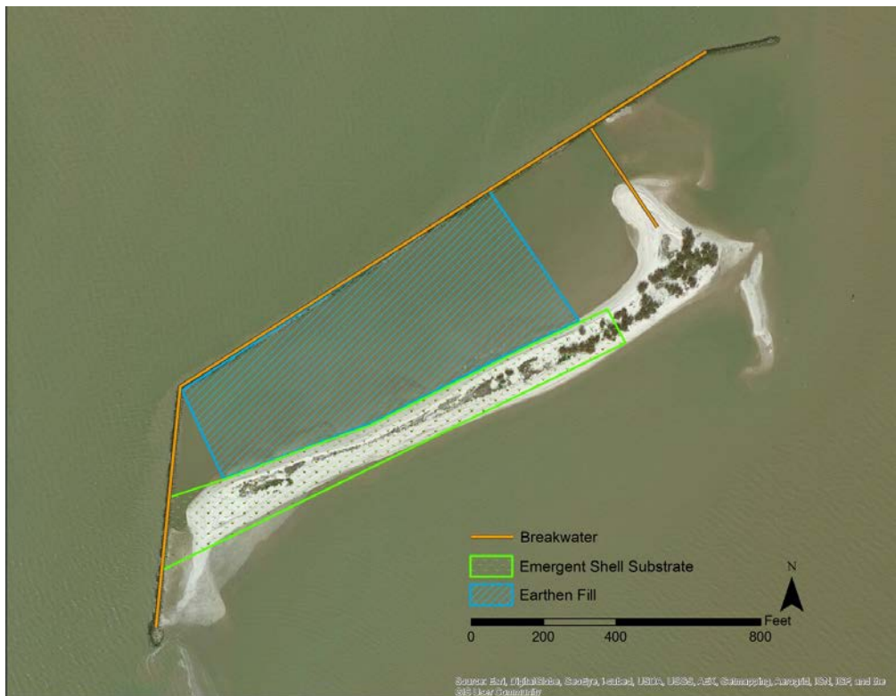
Figure 5-5. Conceptual drawing of the proposed Smith Point Island restoration, illustrating the footprint of the breakwater, fill, and emergent shell substrate
