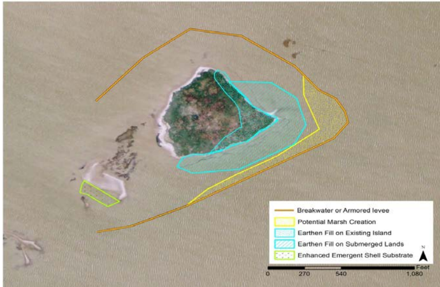
Figure 5-6. Conceptual drawing of the proposed Dressing Point Island restoration, illustrating the footprint of the breakwater/levee, fill, and emergent shell substrate
