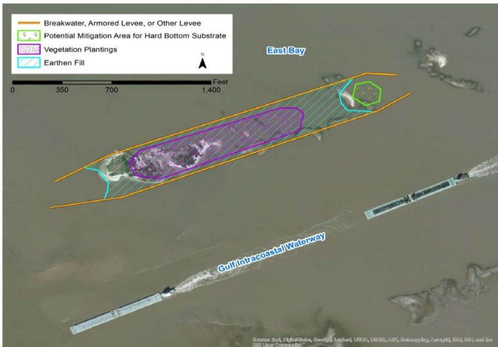
Figure 5-4. Conceptual drawing of the proposed Rollover Bay Island restoration, illustrating the footprint of the breakwater/levee, fill, and vegetation planting area
