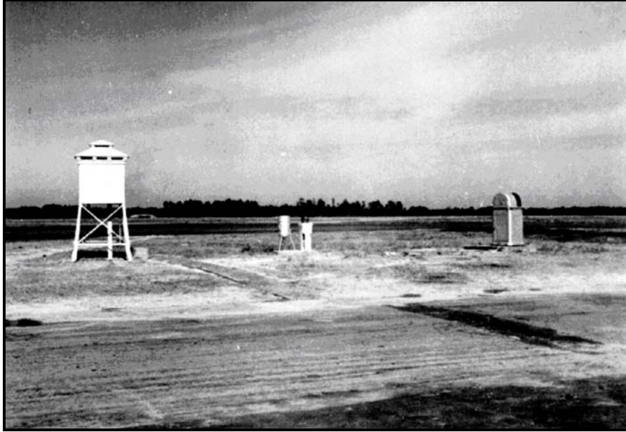
Figure 28. Instrument shelter, standard rain gage, and tipping bucket rain gage (October 1950). View is north. From the official station history files at the National Climatic Data Center.
