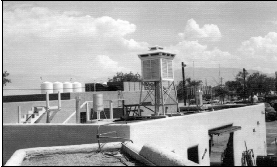
Figure 33. Instrument shelter and rain gages on top the TWA Express Building on 23 June 1958. View is northeast. From the official station history files at the National Climatic Data Center.
