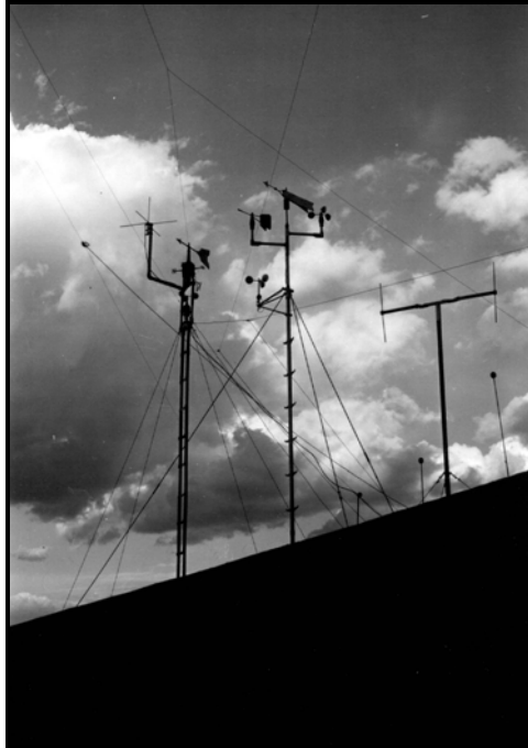
Figure 35. Wind instruments on top of the Administration Building in 1949. Wind instruments on the left belonged to TWA. Wind instruments on the right belonged to the Weather Bureau. The lower anemometer and upper wind vane were wired to the triple register. The upper anemometer and lower wind vane were wired directly to the reading dials in the instrument cabinet in the Weather Bureau office. View is toward the northeast. From the official station history files at the National Climatic Data Center.
