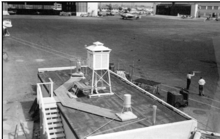
Figure 32. Instrument shelter and rain gages on top the TWA Express Building on 23 June 1958. View is southeast. Weather Bureau note associated with this photograph stated: "Exhaust from parked aircraft common immediately to the right of the instrument group." From the official station history files at the National Climatic Data Center.
