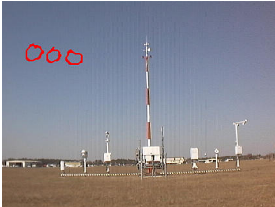
Figure 12. The Automated Surface Observing System at Florence, South Carolina Regional Airport, circa 2000. View is looking north. Source: National Climatic Data Center web site.
