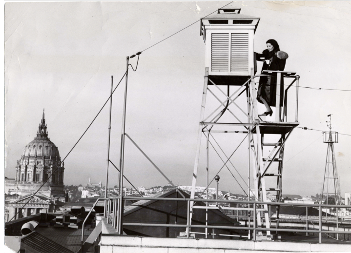
Figure 12. Weather Instrument Shelter, Roof Federal Building, San Francisco Source: With Permission of the San Francisco Public Library
