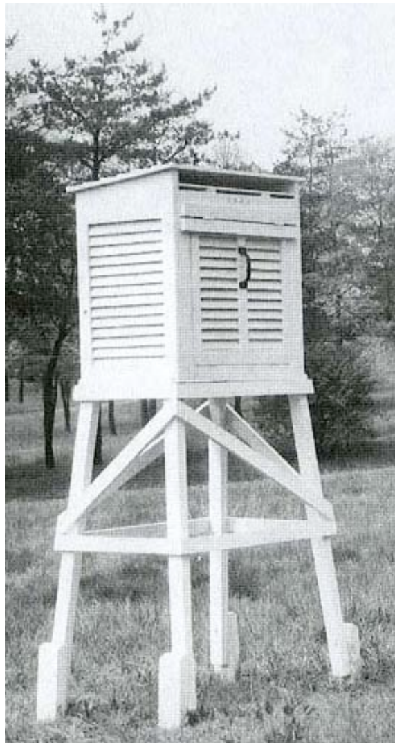
Figure 27. Cotton Region Instrument Shelter of a Type Used in Helena Source: National Archives and Records Administration
