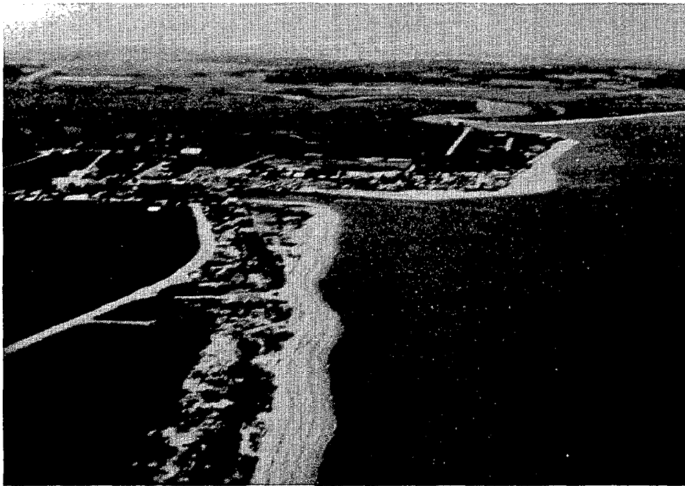
FIGURE 19. Aerial photograph of Bowers and South Bowers looking north. Bowers is situated on a highland between the Murderkill and St. Jones Rivers. The barrier at Bowers is eroding more slowly than the barrier to the south at Bowers Beach which is situated over a deep, pre-Holocene valley now filled with muddy sediments.
