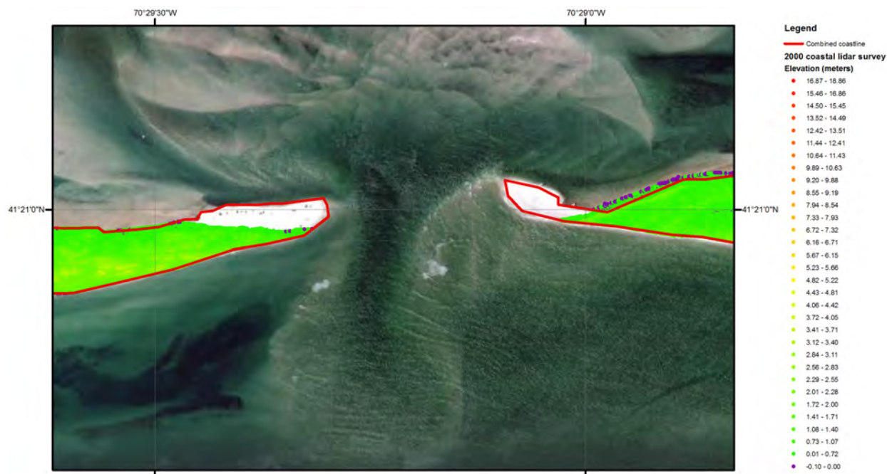
Figure 17. Satellite image of breach in Norton Point Beach. The breach has moved sand northwards into Katama Bay, building two exposed sand bars that were not present during the 2000 topographic lidar survey.
