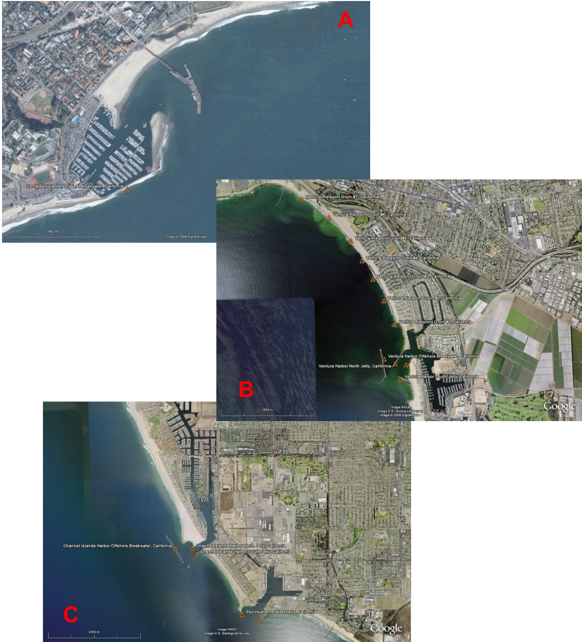
Figure 19. Location of the harbor features digitized by NGDC to represent the jetties and breakwaters shown on Google Earth with USACE overlay of features. A) Santa Barbara breakwater. B) Ventura Harbor jetties and breakwater. C) Port Hueneme and Channel Islands Harbor jetties and breakwaters.
