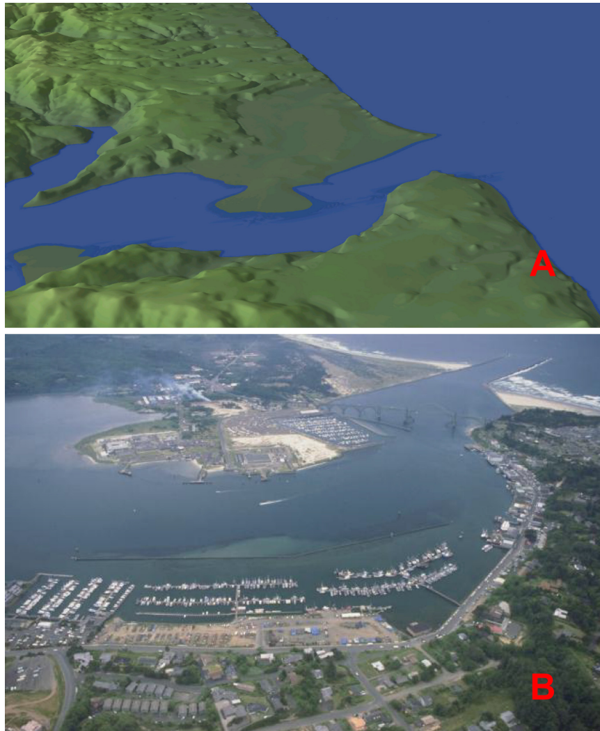
Figure 15. Comparison of the NED 1/3 arc-second DEM shown in QTModeler (A) and USACE aerial photograph (B) of Yaquina Harbor. Note absence of jetties in the NED DEM at mouth of river. Photo from U.S. Army Corps of Engineers Digital Visual Library ( https://portal.usace.army.mil/sites/DVL/default.aspx ).
