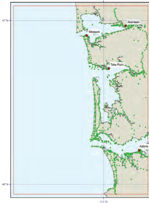
Figure 31. Location of NGS geodetic monuments, shown as green triangles, and the NOAA tide stations, red circles. NGS monument elevations were used to evaluate the DEM.
