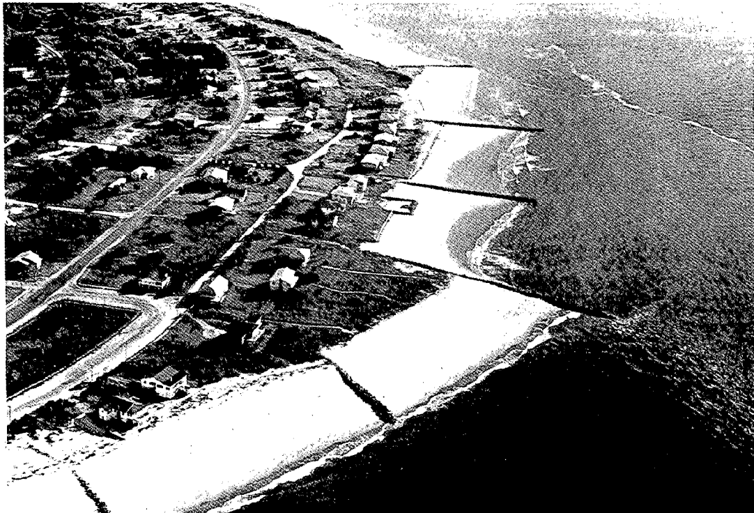
Figure 26. Oblique aerial photograph of a series of groins constructed along Edisto Island beach. Note the accumulation of sand along the updrift (eastern) margin of each groin.
