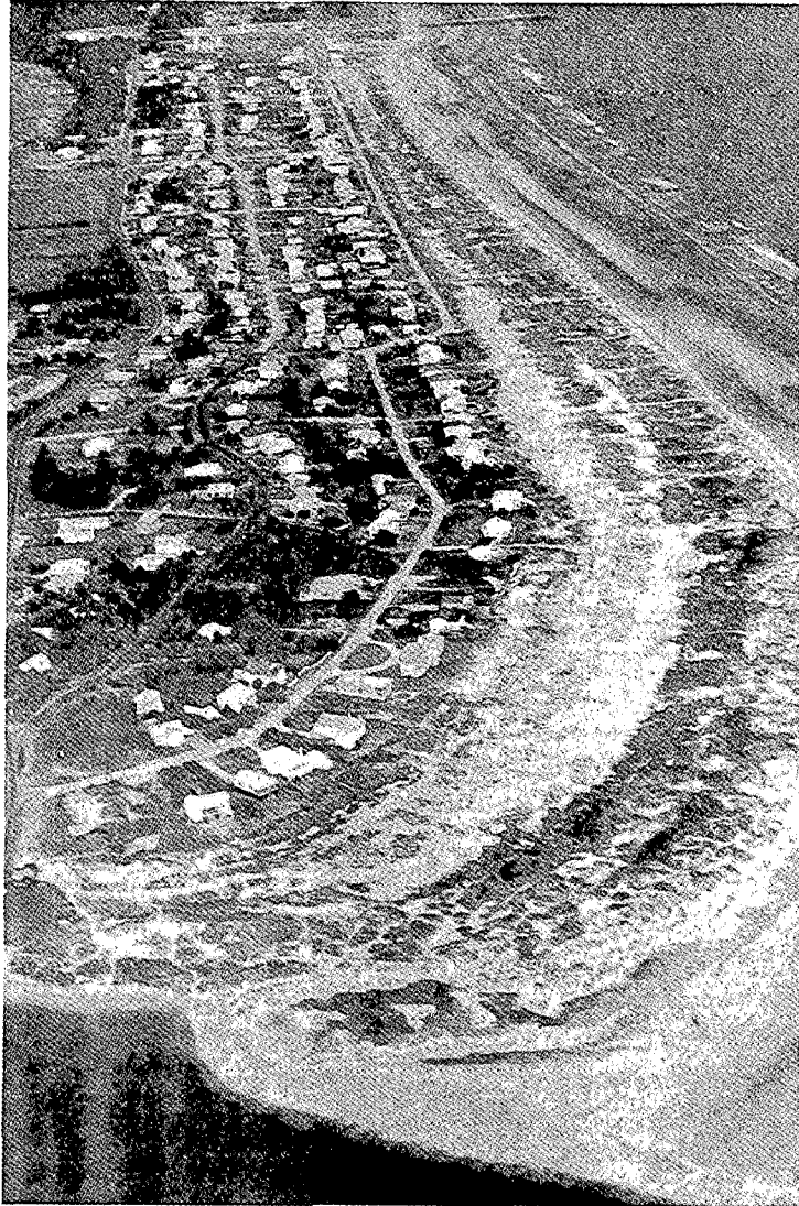
Figure 37. South end of Isle of Palms. Southerly migration of Breach Inlet has allowed the deposition of a recurved spit at the south end of the Isle of Palms. Note houses built on older recurves. Large open area is where a developer has flattened the sand dunes in the location of profile stations IP-03 and IP-04. View looks north.
