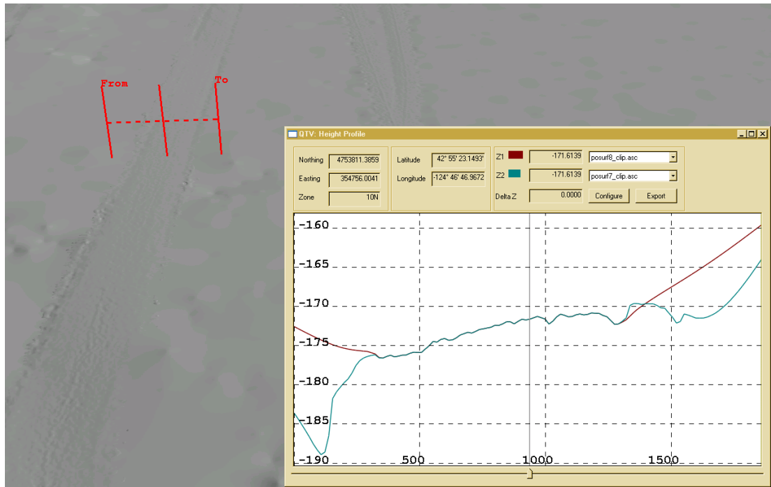
Figure 11. QT Modeler image of cross section comparing gridded bathymetric surfaces of pre-edited data (shown in blue on the graph) and the post edited data (shown in red on the graph).
