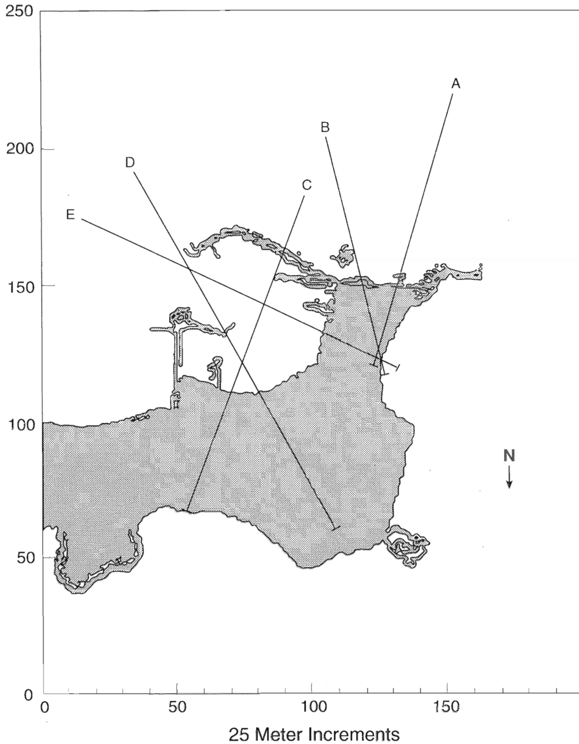
Fig. H-3. The Crescent City inundation areas for a 10-m, 33.3-min-period high tsunami. Lines labeled A, B, C, D, and E represent the locations of the engineering model used to cross check the inundation model calculations. The length of the line represents the extent of flooding estimated by the engineering model.
