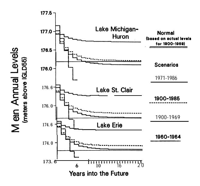
Figure 7. --Mean annual water levels of Lakes Michigan-Huron, St. **Clair**, and Erie resulting from **scenarios** of low and moderate water supplies.
