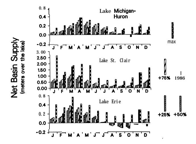
Figure 9. --Monthly net basin supplies to Lakes Michigan-Huron, St. Clair, and Erie used in simulations of rising lake levels.
