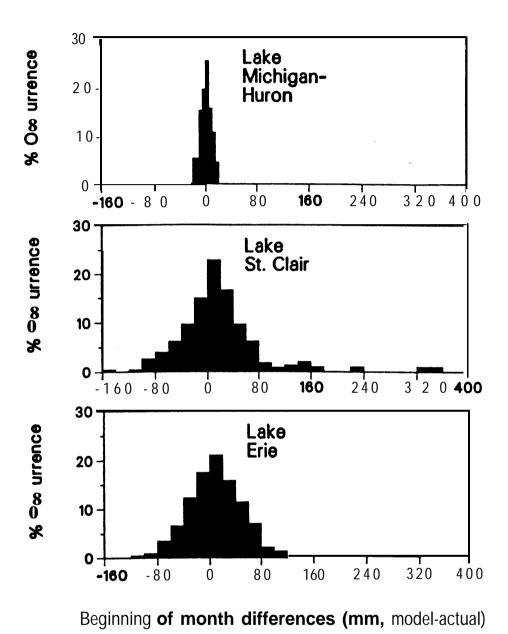
Figure 1. --Deviation **between** modeled and actual beginning-of-month lake levels
