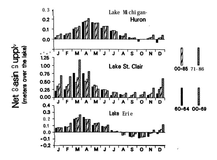
Figure 6. --Monthly net basin supplies to Lakes Michigan-Huron, St. Clair, and Erie used in simulations of falling lake levels.
