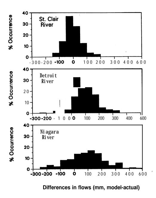
Figure 2. --Deviation between modeled and actual monthly connecting-channel flows for the calibration period.
