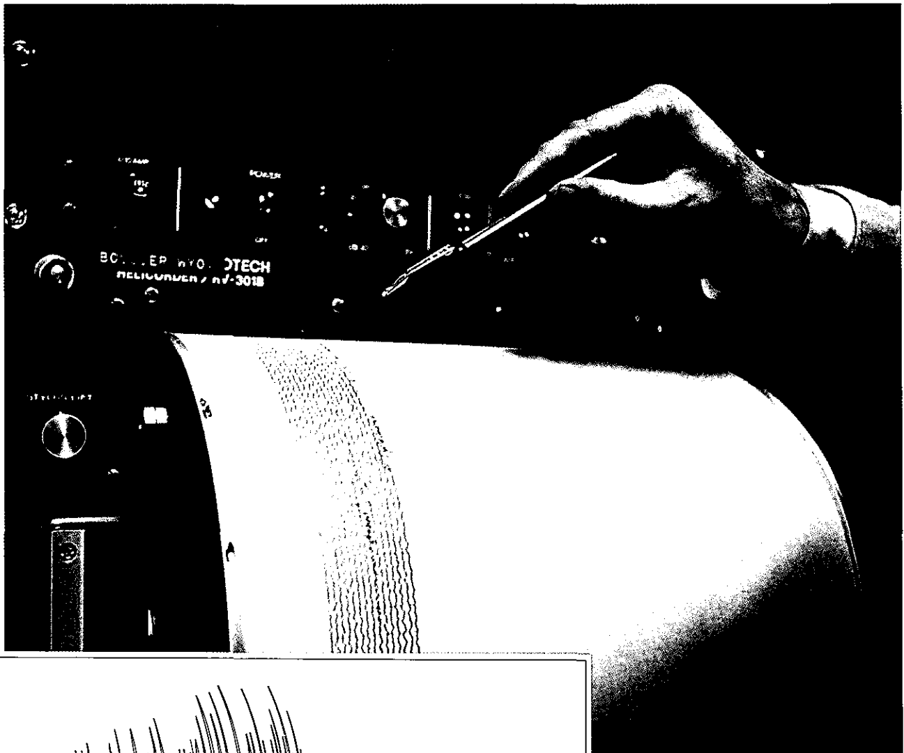
A modern seismograph records Earth motions on a strip chart such as the one below the photo. This seismogram shows the trace made by the August 6, 1979 California earthquake. Credit: Dr. Henry Spall U.S. Geological Survey
