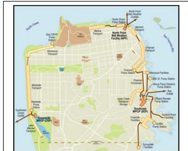
Figure 16 San Francisco combined sewer system transport and storage boxes (from San Francisco 2030 Sewer System Master Plan 2011)
