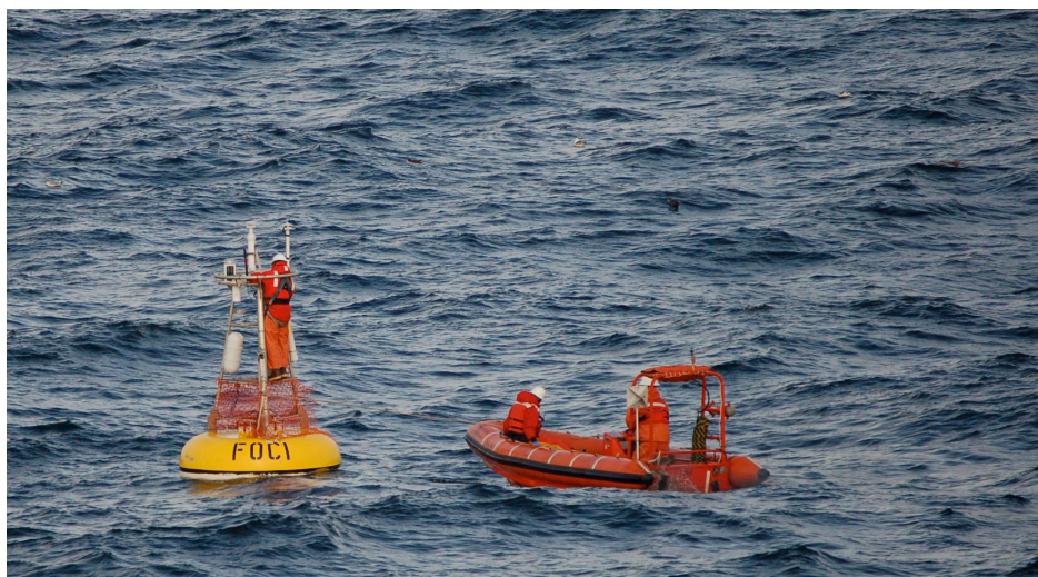
EcoFOCI personnel service the M2 mooring, which has (as of 2013) collected year-round temperature, salinity, nitrate, chlorophyll, current, and sea ice measurements in the Bering Sea for 19 consecutive years
