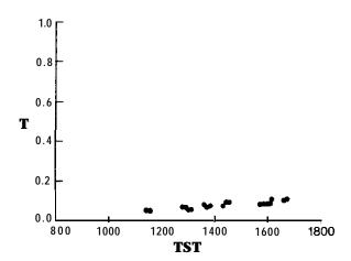
Figure 17. Increase in radiation transmittance due to snowmelt as indicated by the rise in transmittance ratio (T) with true solar time (TST), 22 February 1977.
