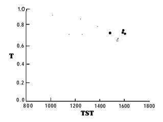
Figure 20. Transmittance (T) versus true solar time (TST) showing differences in (T) due to cloud-cover variability for 18 January 1977.
