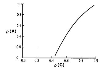
Figure 28. Upper layer reflectance,  $\rho(A)$ , versus combined transmittance,  $\tau(C)$ , and upper layer reflectance,  $\rho(A)$ , versus combined reflectance,  $\rho(C)$ , from operation of the two-layer model for a situation where the underlying layer simulates snow ice.
