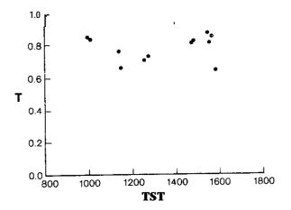
Figure 15. Radiation transmittance (T) versus true solar time (TST) during a period of variable cumulus cloud coverage and during periods between depth profiles for 7 January 1977.
