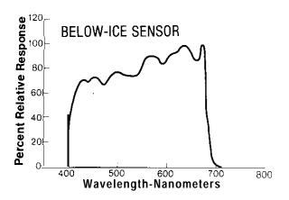
Figure 3. Relative spectral response of the two sensors used in this study.
