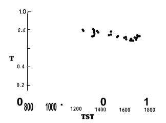
Figure 13. Radiation transmittance (T) as a function of true solar time (TST) during ice decay for 8 March 1977.
