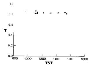
Figure 18. Ratio of under-ice to incident radiation (T) versus true solar time (TST) on a partly cloudy day with a changing ice surface, 6 January 1977.
