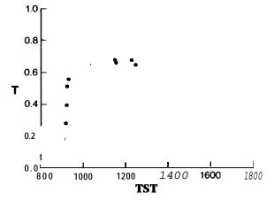
Figure 9. Ratio of under-ice to aboveice radiation (T) versus true solar time (TST) as the ice surface was progressively cleared of a thin snow layer, 26 January 1977.
