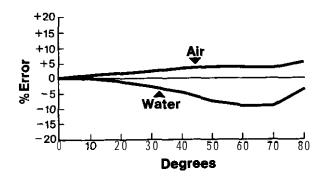
Figure 4. Cosine response of typical underwater sensor (from Roemer and Hoagland, 19771.
