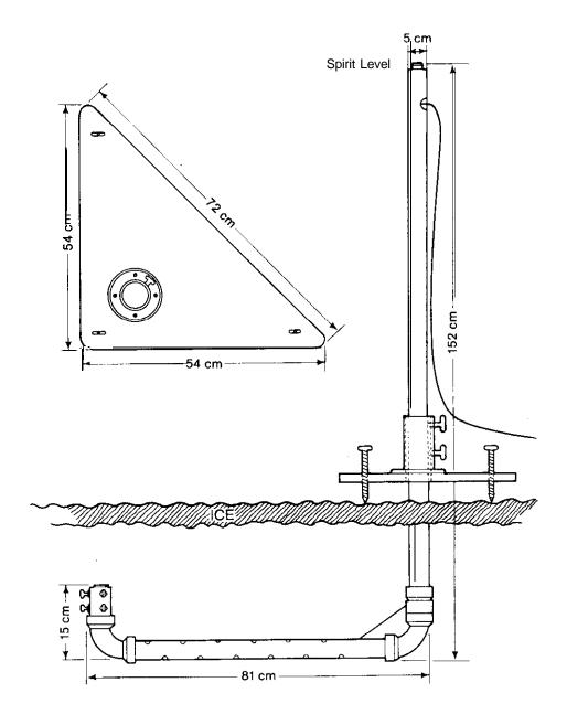
Figure 5. Design details of the support am for the underwater sensor.
