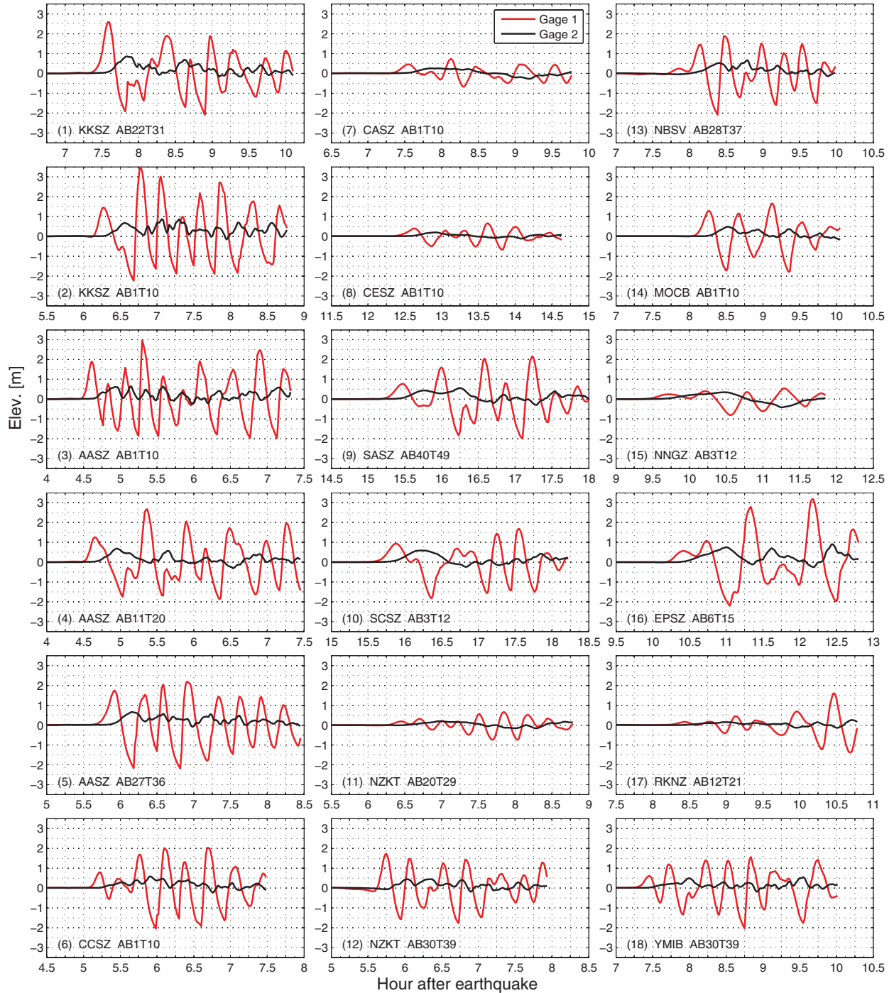
Figure 19: Comparisons of computed wave amplitude at the open coast (Gage 1) and Ford Island (Gage 2) for 18 simulated M_w 9.3 tsunamis. Results are from the 1'' test model.
