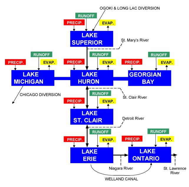
Figure 5. Arrangement schematic of Great Lakes, connecting channels, and all water flows.
