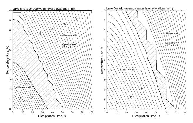
Figure 12. Steady state lower Great Lakes average water levels as a function of temperature rise and precipitation drop relative to the present base climate.
