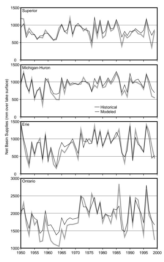
Figure 6. Net basin supply comparison for 1950-1999 of observed (historical) and simulated (modeled) supplies.
