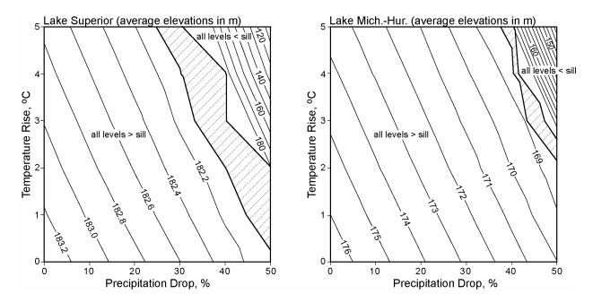
Figure 11. Steady-state upper Great Lakes average water levels as a function of temperature rise and precipitation drop relative to the present base climate.
