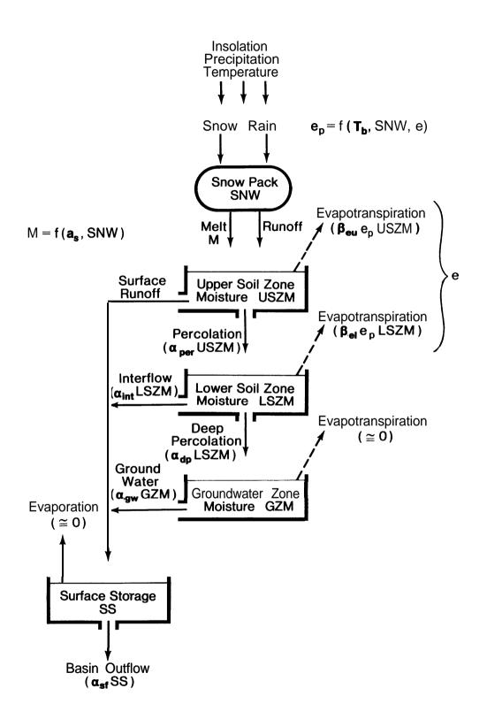
Figure 1. -- Conceptual schematic of large basin runoff model.
