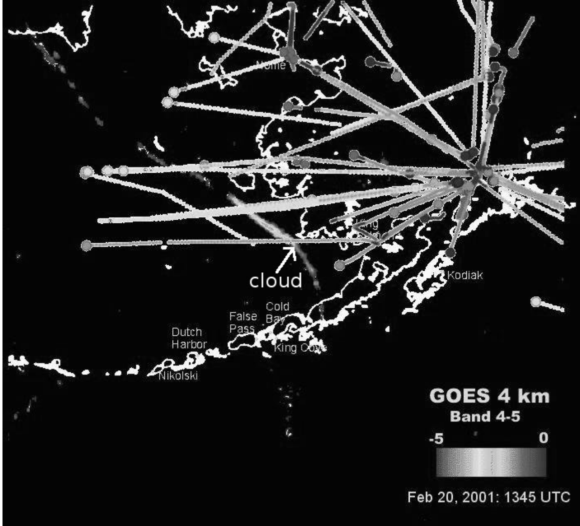
Figure 1 – Composite GOES brightness temperature difference (BTD) image at 1345 UTC on February 20, 2001 overlaid with all flight routes at 1345 \pm 30 minutes. The last recorded position of each flight is shown with a filled circle. Most all flights are entering or leaving Anchorage Int'l Airport. The ash cloud as detected using BTD is shown just slightly off of the west coast.
