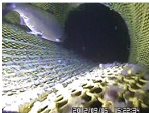
Figure 28. Escapement out the top portion of the excluder during Pacific Prince EFP
