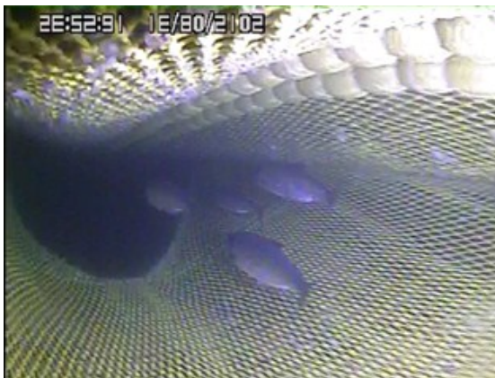
Figure 27. Several salmon escaping from bottom excluder seen from port side camera
