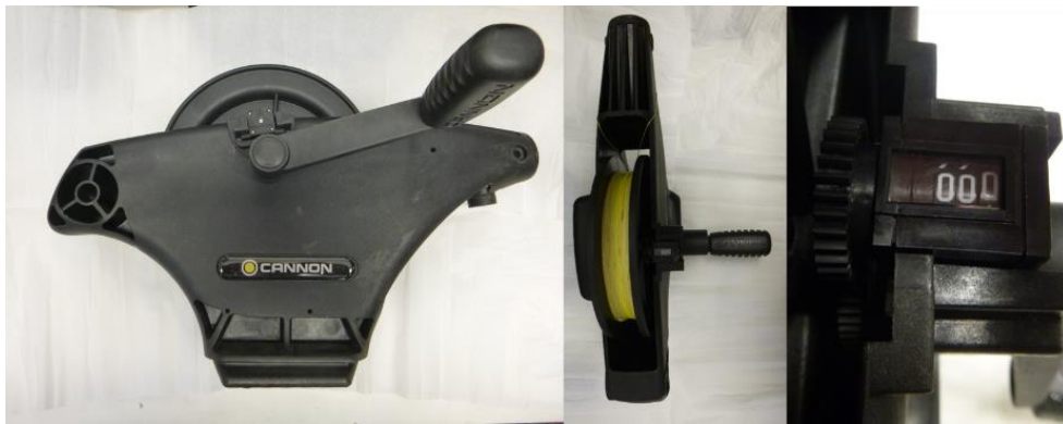
Figure 3. Detail of deep sea reel ('downrigger') and counter.
